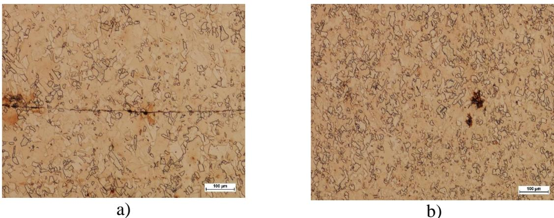
Figure 4 – Sample images of the microstructure of deformed samples in the area of the connection zone: (a) at 540°C and 10 mm reduction in length, (b) at 640°C and 10 mm reduction in length
